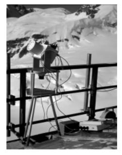
Figure 2 Reagan solar radiometer with 10 spectral bands between 382 and 1033nm during a high altitude calibration campaign.
