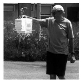
Figure 1 Radiosonde for air pressure, temperature, humidity, wind, and ozone sounding.
