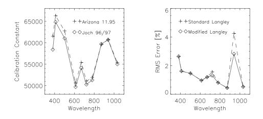
Figure 3 Calibration constants determined at Mount Lemmon (1995), at Jungfraujoch (1996), and Weiss-fluhjoch (1998); derived by the modified Langley plot method.
