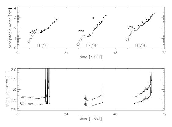
Figure 7 Top: Precipitable water measured by radio sondes (asterisks) and by the solar radiometer (solid line) at Grono. August 16 - 18, 1996. Bottom: Optical thickness of the radiometer channels 1 (381 nm) and 3 (501 nm).
