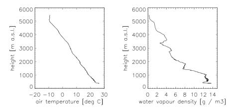
Figure 5 Typical temperature and water vapor density profile on a clear summer morning.
