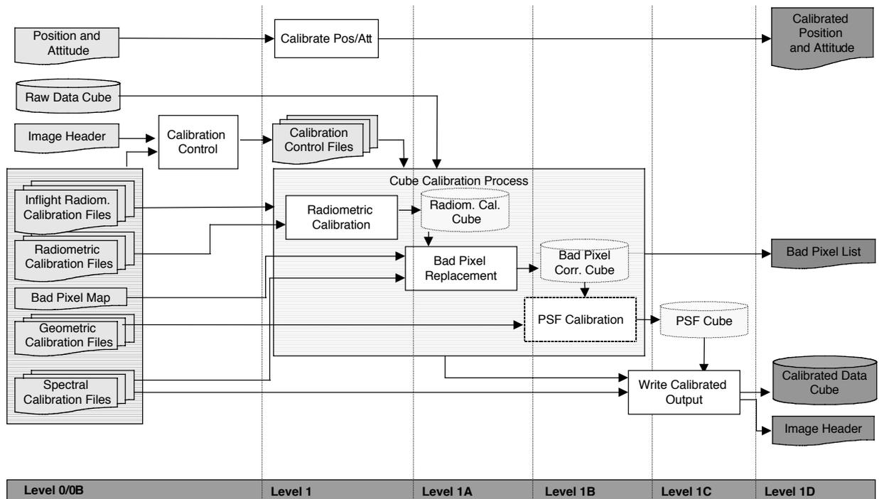
Figure 3. Level 1 Processing Concept
