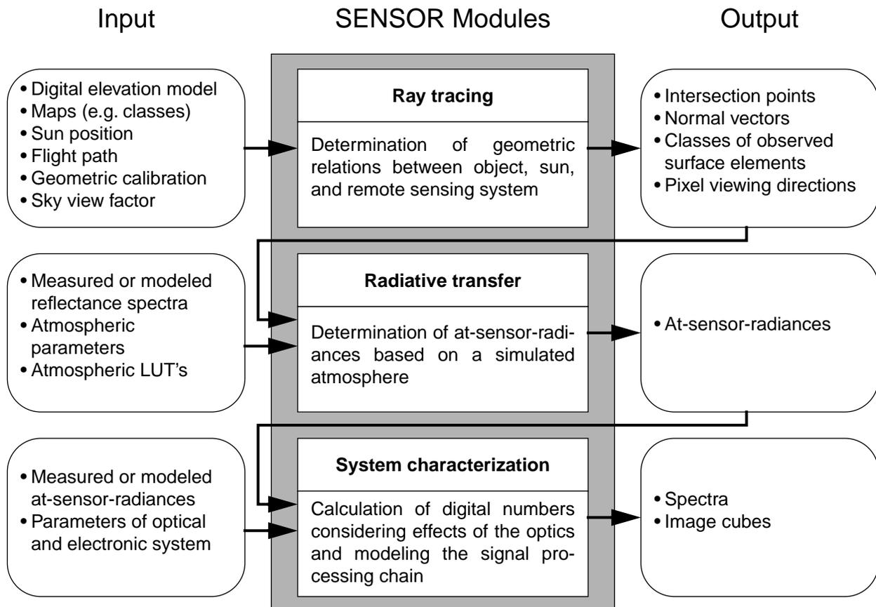
Fig. 2: Scheme of the software environment for the simulation of optical remote sensing systems (SENSOR)
