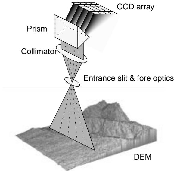
Fig. 1: Principle of a pushbroom imaging spectrometer using a prism
