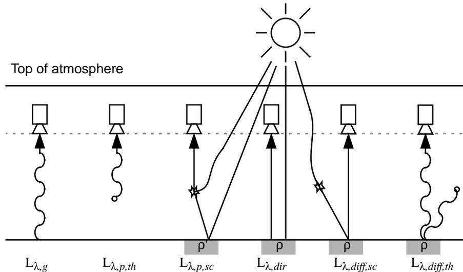
Fig. 5: Contributing parts of total at-sensor-radiance (after Wiest, 1998)
