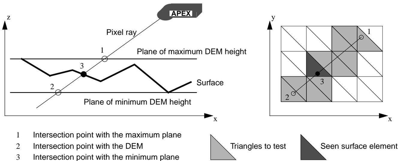
Fig. 4: Principle of ray tracing in a digital elevation model, side view (left), top view (right)
