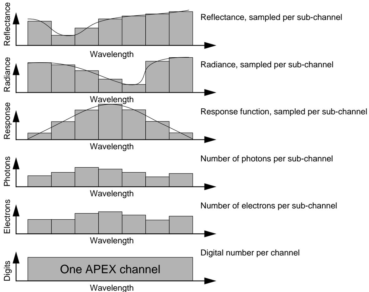
Fig. 6: Sub-channel concept for signal generation within SENSOR
