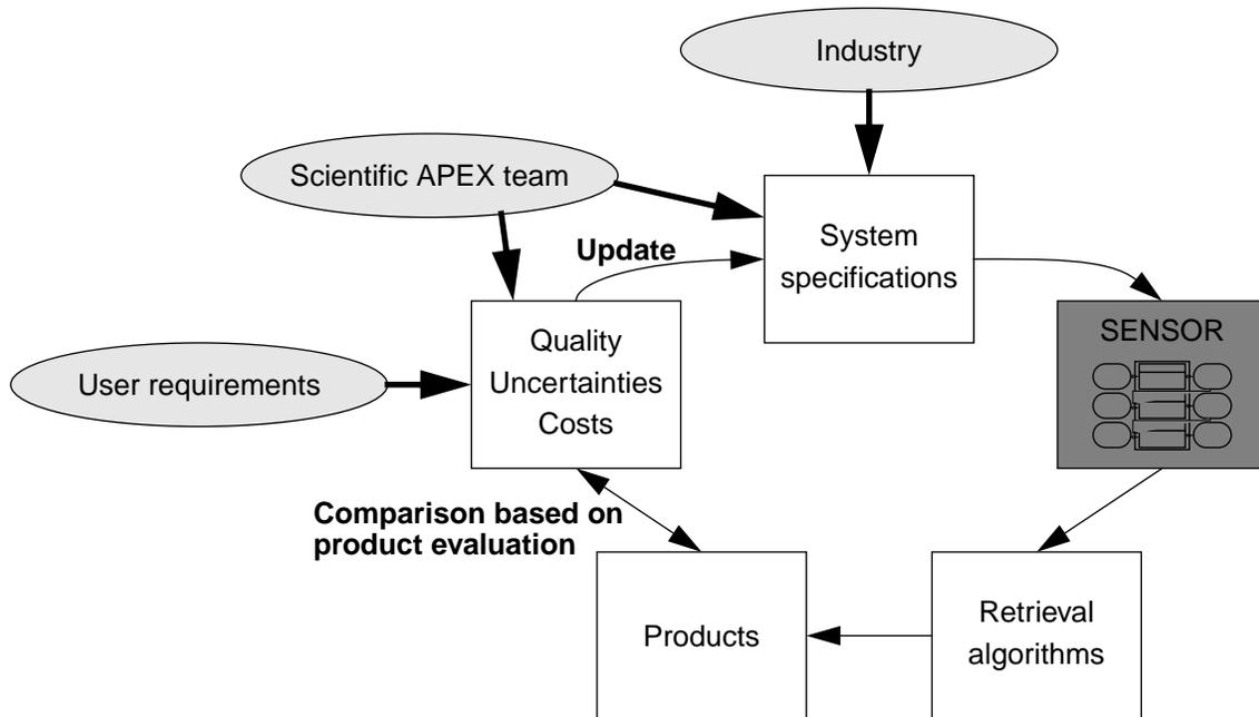
Fig. 9: General scheme for an optimization or evaluation process using SENSOR
