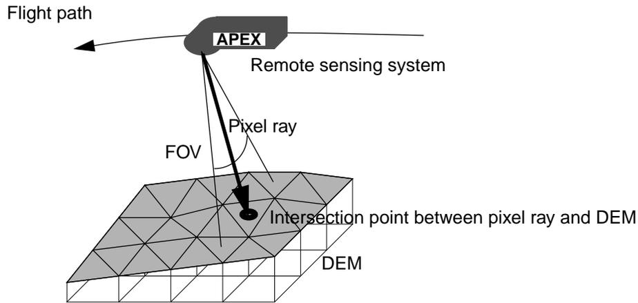
Fig. 3: Ray tracing in a digital elevation model
