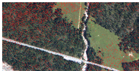
Figure 6: Influence of surface model preprocessing on geometric accuracy: red pixels are shifted in position if a 3x3 smoothing filter is applied to the DSM before geometric processing.
